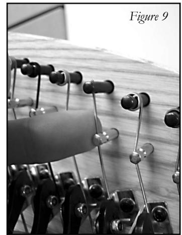
8. Pinch the string against the tuning pin as the string is being wound. This puts some tension on the string and gives it tight, even coiling. You want the coils to lie evenly side by side (*figure 10*).
