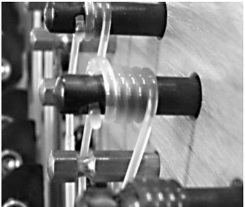
*Figure 5: Tuning pin, bridge pin, and sharpening lever*
